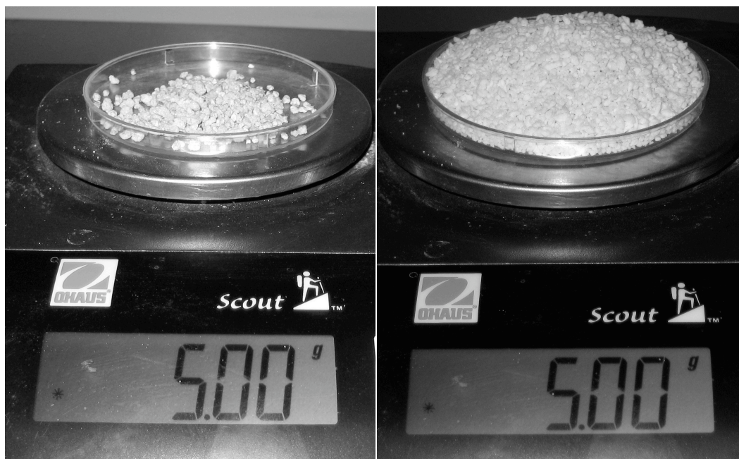
Figure 10.8. Difference in volume of 5 g unexpanded perlite (left) and 5 g expanded perlite (right).
