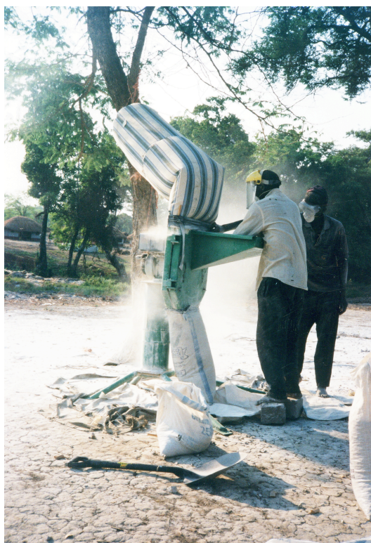
Figure 7.10. Demonstration of the mobile locally produced modified hammer mill, used to grind local limestones in Zambia. (Photo, courtesy of Prof. S. Simukanga).
